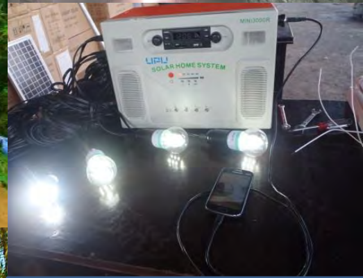
30-Wp Solar Home System
