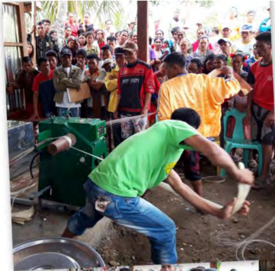
Solar powered abaca spindler New Mabuhay, Malita, Davao Comissioned by ASEP Experts October 2018
